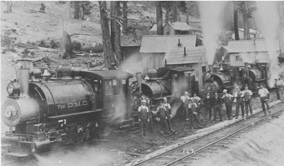
Line-up of meter gauge locomotives 6, 1, 2, 4 and 3 at Ramsey Bar camp of the Diamond Match Company.
