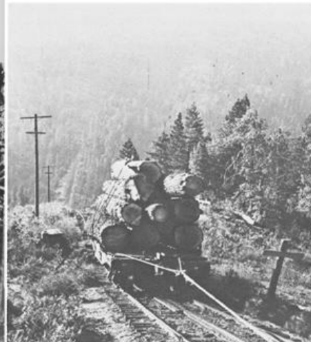
Changing cables in the "hole" at the bottom of the inclines. The loaded car at right has arrived from the west side, the empty flat from the east. The cables will be switched on the two cars, which will then continue their respective ways. The car (below) nears the top of the east side.
