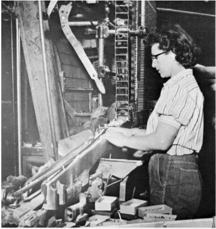
SAW (strike anywhere) kitchen matches being boxed by an automatic packer in the Chico factory in 1957. The Chico factory had eight of these machines at that time (photo courtesy Diamond International Corporation).
